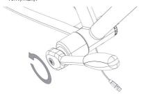
7. Fasten the lock cap on non chain wheel side clockwise with special tools. Tightening torque requirement: 30 Nm(max).
